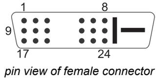
\* Hot plug detect (HPD) is fully DVI compliant. DVI sources detect the presence of a display device by providing +5V on pin 14 and looking for +5V on pin 16. Whenever the projector is operational, and 5V is present on pin 14, pin 16 will be held at +5V.
