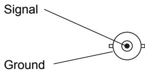
SMPTE 292 / HD-SDI signals are very high speed digital signals which require better quality coaxial cable than conventional analogue video. The data rate is 1.5 Gigabits per second.
